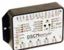
The **Atkinson GSCM** (generator start controller module) is a microprocessor-based generator-starting controller that receives start commands from any 12 VDC output or dry-contact switch, including an inverter or charge controller auxiliary relay, a voltage controlled relay, a timer, a water tank float switch, or any user-supplied contact closure. It automatically controls a gas/propane or diesel powered generator or pump, and is sealed for harsh environment operation.
