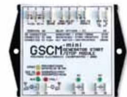
This **GSCM-mini** generator start controller is optimized for use with OutBack inverters. It supports three types of 3-wire gas-generator control: momentary, maintained, or ignition. It has a fixed crank time and over and under frequency shutdown. 2-year limited warranty.
